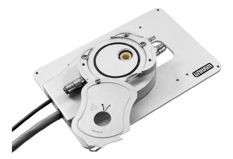
**Rapid Heating Rates** From ambient to 1500°C at a rate of up to 150°C/min **High Temperature** Accurate temperature control between ambient and 1500°C **Rotating Quartz Window** Continuous sample observation and high resolution imaging
