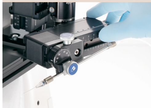
Swivel out function for easy capillary exchange.
