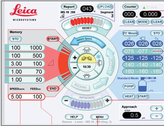
Counter window to toggle between section counter and feed totalizer, countdown, E-W measuring, and AutoTrim mode.
