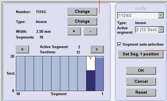
To optimize diamond knife usage, up to 100 different knives can be stored. Each knife is divided into a number of segments. The selected segment is approached automatically with the motorized knife stage (patent applied).
