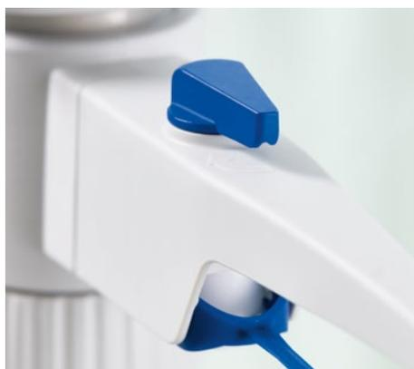
Recirculation valve lever for easy setting of recirculation or dispensing position
