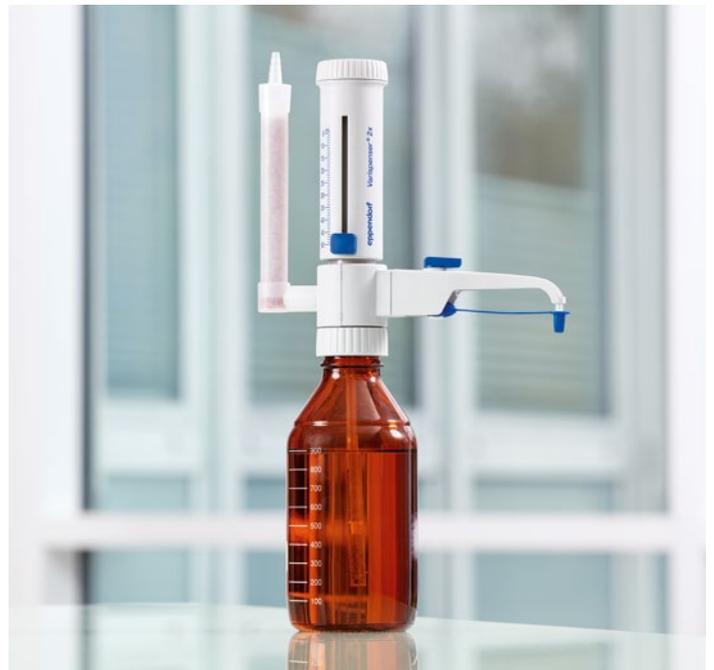
E.g. fuming acids often used in chemical industry need to be kept free from moisture. The drying tube – filled with moisture absorber protects the liquid.
