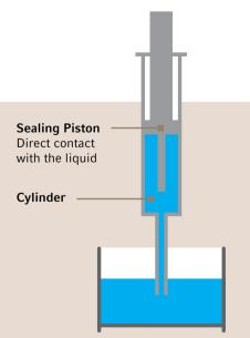
Learn more about handling non-aqueous solutions and the Multipette system at: www.eppendorf.com/multipette-system
