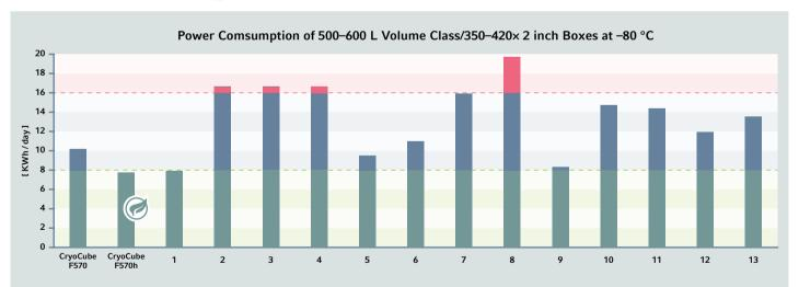
A comparison of the number of kilowatt hours per day it takes to keep 350 - 420 individual 2 inch boxes at a temperature of -80 °C in freezers with a volume of 500-600 L. The CryoCube F570h (230 V/50 Hz) can maintain the storage temperature using 7.6 KWh/day, less than 50 % of the energy required by some other units.
