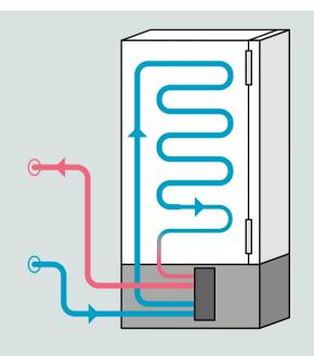
You can improve the conditions and comfort in your lab while saving energy by installing a water-cooled Eppendorf freezer. Many ULT freezers use the air in the laboratory to extract heat energy from the freezer's heat exchanger. Another option is to use a water-cooled ULT freezer connected to a facility's recirculating water system. A constant stream of water removes the heat from the heat exchanger, rather than the ambient air in the lab.
