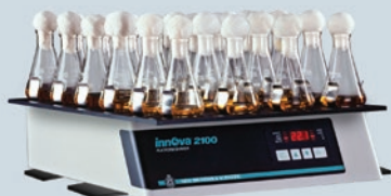
Innova 2150 Maximum flask size: 6 L Orbit: 1.9 cm (0.75 in)
