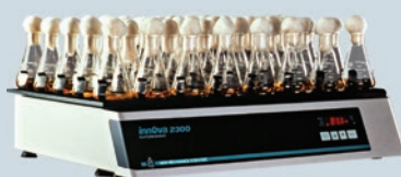
Innova 2300 Maximum flask size: 6 L Orbit: 2.5 cm (1 in) or 5.1 cm (2 in)
