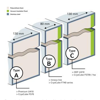
Eppendorf offers three varieties of insulation design. You can choose the design that meets you energy-saving, capacity, and cost parameters.
