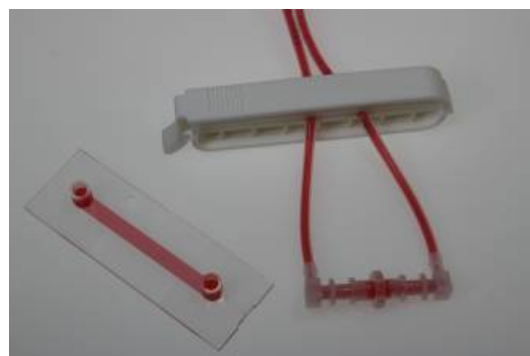
Figure 31: Clamp the tubing before opening the Female Luer Coupler of the Perfusion Set.
