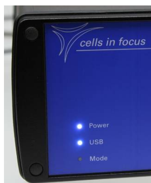
Figure 17: LEDs on the pump’s front panel indicating the connected USB and power supply.
