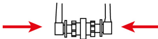
Figure 21: Secure the Luer adapters in the Female Luer Coupler.
