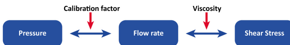
Figure 36: Influence of the calibration factor and viscosity on the parameters of the PumpControl software.
