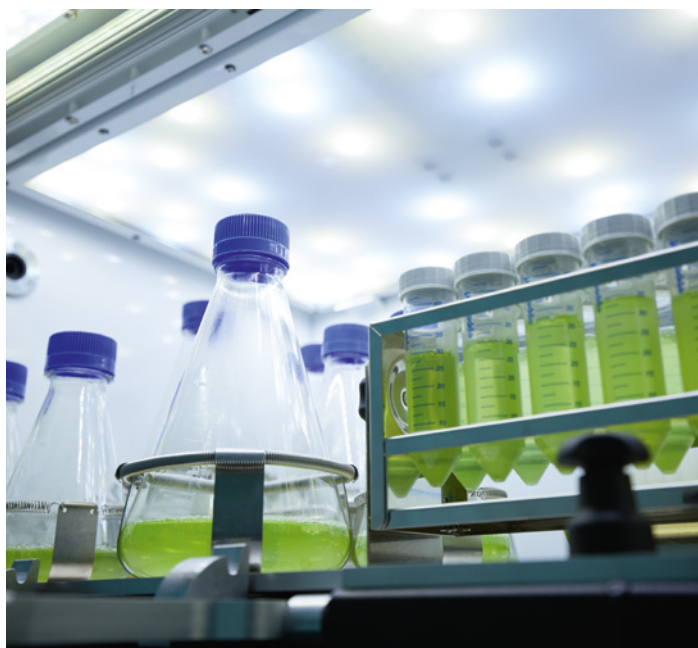
Grow phototrophic cells using integrated photosynthetic LED lights
