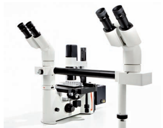
Discussion attachment for two observers on the Leica DM IL LED
