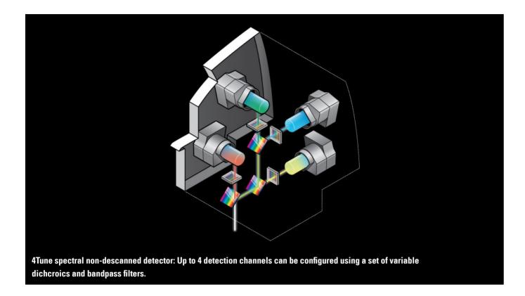
At the heart of STELLARIS 8 DIVE is 4Tune, the first and only spectral non-descanned detection system. Through a combination of state-of-the-art non-descanned detection – the most sensitive way to collect scattered signals from deep layers – with a set of variable dichroics and bandpasses, deep in vivo multicolor imaging becomes possible.
