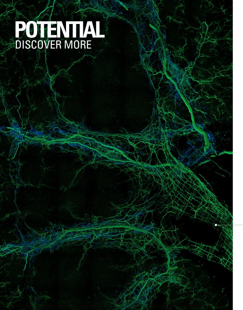
The integration of TauSense in STELLARIS 8 DIVE enables you to image tissue structures or study metabolic changes, such as changes in the NAD/NADH ratio, without the need of additional staining. This saves you the time and effort of labeling steps and allows the monitoring of components that cannot be labeled without perturbing their function, such as NADH.
