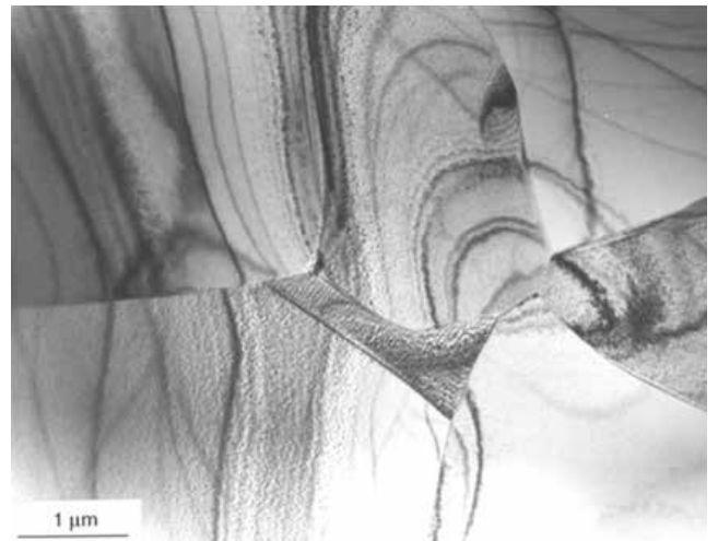
STEM images of a Ti film that has been ion beam milled at an angle of 6°
