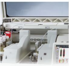
The first and only workstation in the market with dual glass coverslip lines enabling the highest throughput of up to 570 dried slides per hour.
