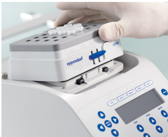
SmartBlock removal from Eppendorf ThermoMixer® C
