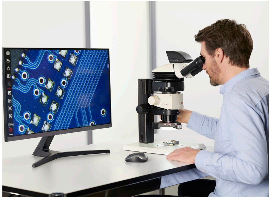
M60 stereo microscope with Flexacam c5 camera using the on-screen display (OSD) of the Enersight software platform.
