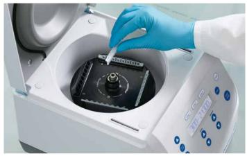
Centrifuge 5420 offers two rotor options: A 24-place standard rotor for up to 24 x 1.5 or 2.0 mL tubes and a PCR-tube rotor for  $4 \times PCR$  strip or  $32 \times PCR$  tubes (0.2 mL).
