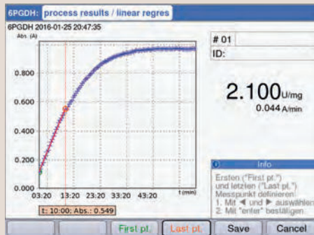
Linear regression analysis of an enzyme activity measurement with adjustment of start and end point.
