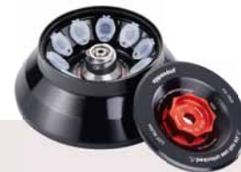
Aerosol-tight Eppendorf QuickLock® rotor for 10 × 5.0 mL tubes * spins up to 21,330 × g /15,060 rpm; accommodates adapters to hold 1.5/2 mL, HLPC, and Cryo tubes (FA-10 × 5)
