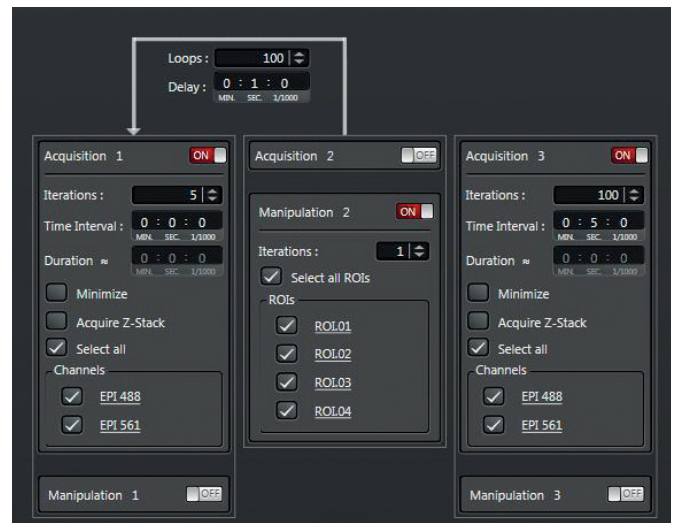
Add and configure experiments using the flexible experiment design tool in LAS X software.
