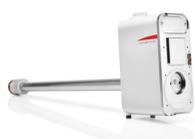
The EM FC7 can be outfitted with an EM VCT500 to transfer environmentally sensitive and / or cryogenic samples.
