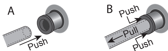
Figure 2: How to connect and disconnect the gas tubing to the push-in fittings of the ibidi Air Pressure Generator and the ibidi Gas Mixer. Push in to connect (A). Push and pull to disconnect (B).
