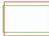
For live imaging, the Leica DMS300 has an image detail in 16:9 format on an HD-monitor (displayed with a green frame). The images are always saved in a 4:3 size ratio (shown with a red frame).
