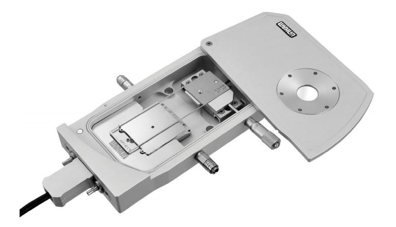
**Temperature Control** T96-P LinkPad controller allows fast and accurate temperature programming **Thermoelectrically Cooled** Cooling below ambient temperatures without the need for liquid nitrogen
